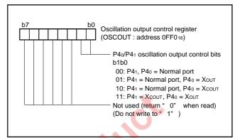
Fig. 54 Structure of oscillation output control register
