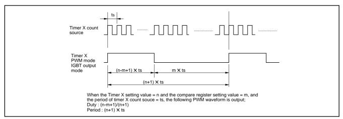
Fig. 22 Waveform of PWM/IGBT
