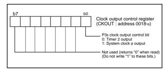
Fig. 45 Structure of clock output control register
