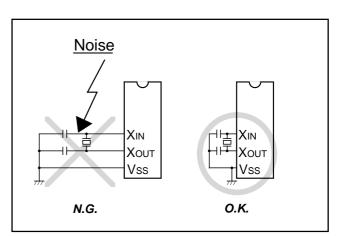
Fig. 57 Wiring for clock I/O pins
