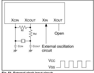
Fig. 51 External clock input circuit
