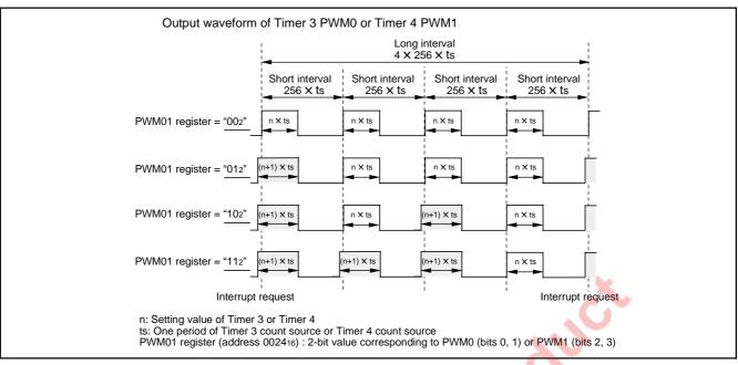
Fig. 21 Waveform of PWM0 and PWM1
