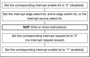
Fig. 5 Sequence of changing relevant register
